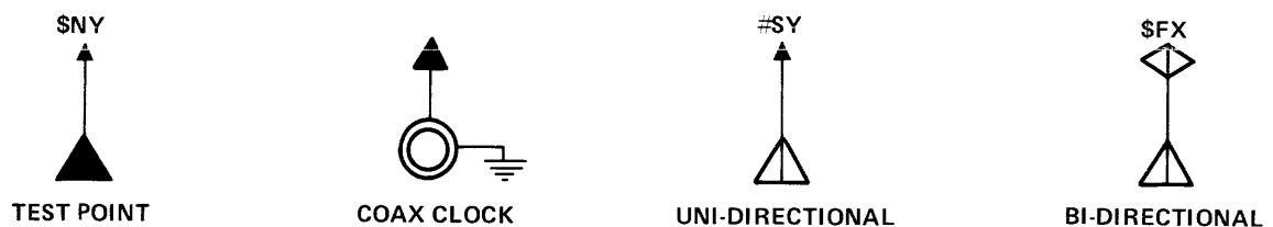
Figure 3-2. Schematic Backplane Pin Symbols
